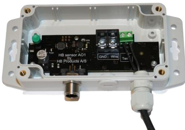
The temperature sensor is mounted in the box at delivery. The Sensor wire can be demounted/mounted/replaced using the green connector named "Ten". The large black connector named GND and Wire is not used.
